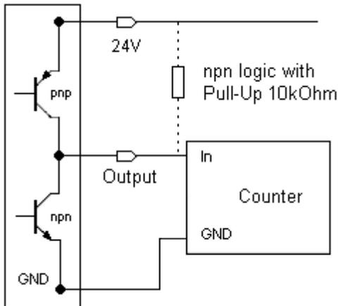
Fig.12: Connecting output 1 to external counter
