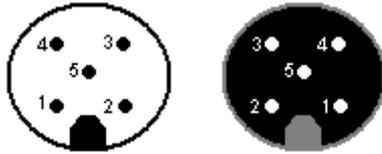
Fig.7: Pin code: Connection plug / socket
