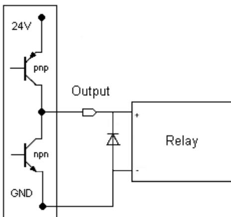
Fig.13: Connecting output 2 to relay
