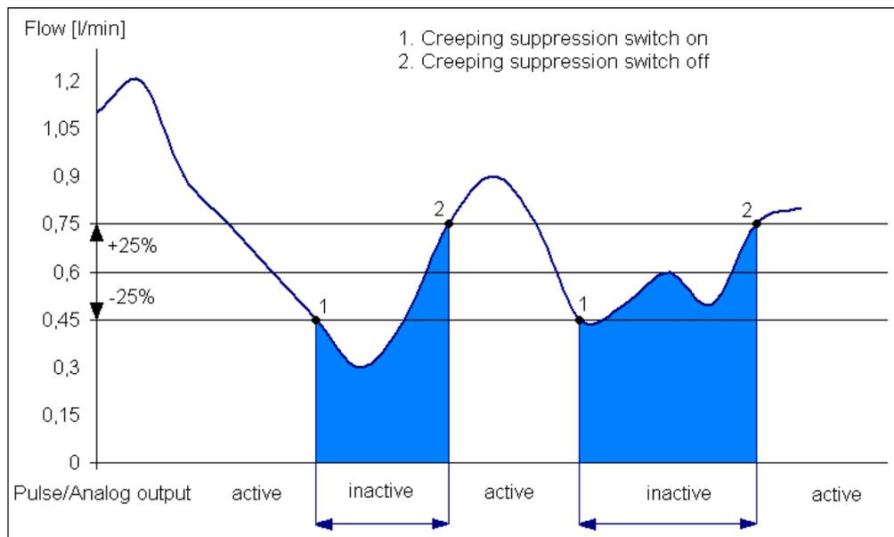
Fig.11: Function of the creeping suppression illustrated with 0.6 l/min
